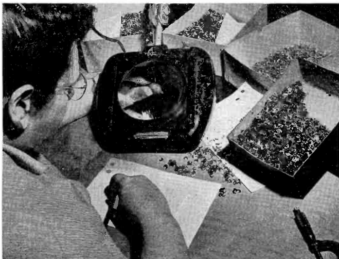
Tiny tube parts are magnified and their outlines superimposed on scale drawings to insure meeting the extremely close tolerances required.
